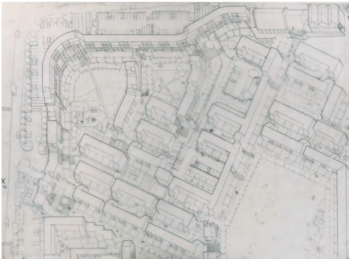
18. Axonometric projection of the north-west corner showing the relationship between the Wall, public spaces and low-rise housing.
