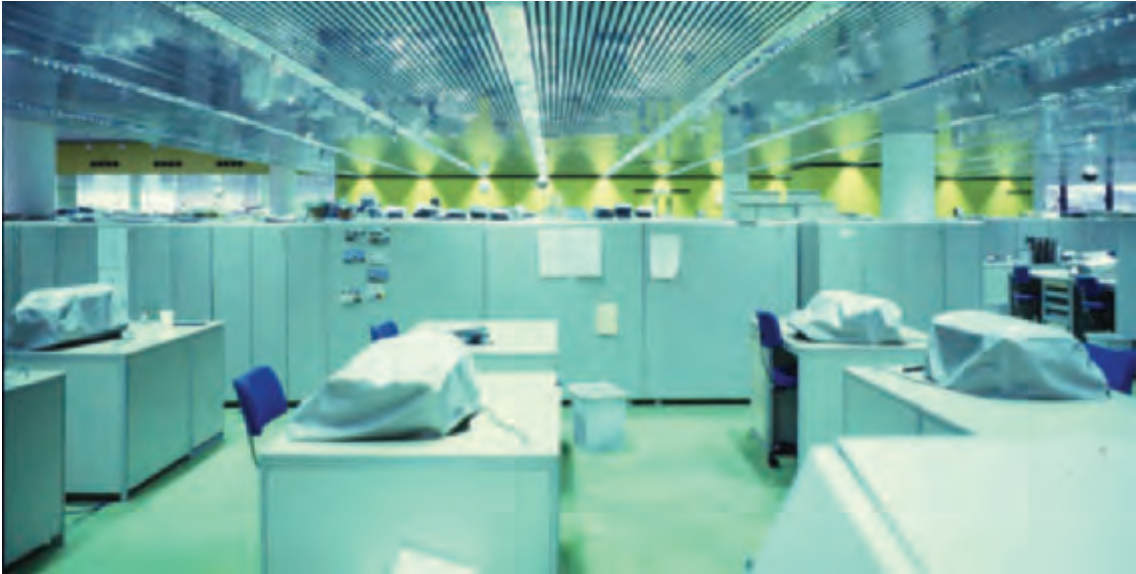
18. Typical deep-plan office with artificial lighting and ventilation in the ceiling, cabling under the floor, allowing flexibility of office layout.
