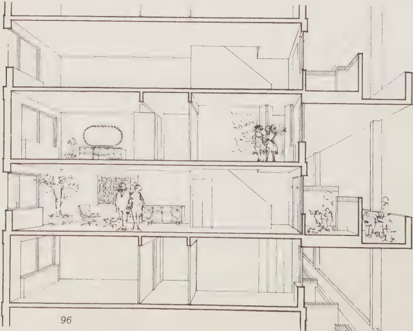
101. Riverbend Houses. Section perspective, showing typical duplexes with "front porch" and "street in the sky."
