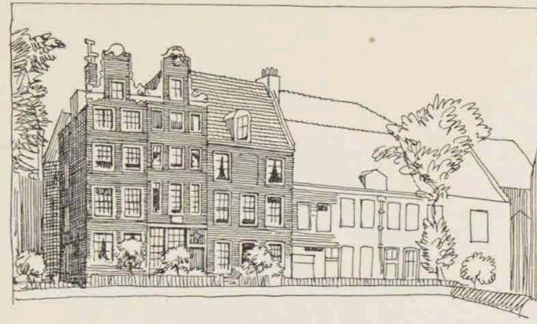
Houses at Begijnhof in Amsterdam. The two houses to the left with the typical "halsgevel" breaking through the horizontal cornice of the Baroque façade.
