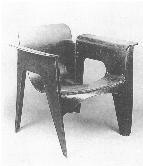
30 'Birza chair', designed in 1927 for the Birza apartment; made from a single sheet of shaped fibre held in place with a series of nuts, bolts and washers. Van de Groenekan refused to make any more because of the difficulties of construction. Apparently the fibre was soaked in water and modelled on a bench
