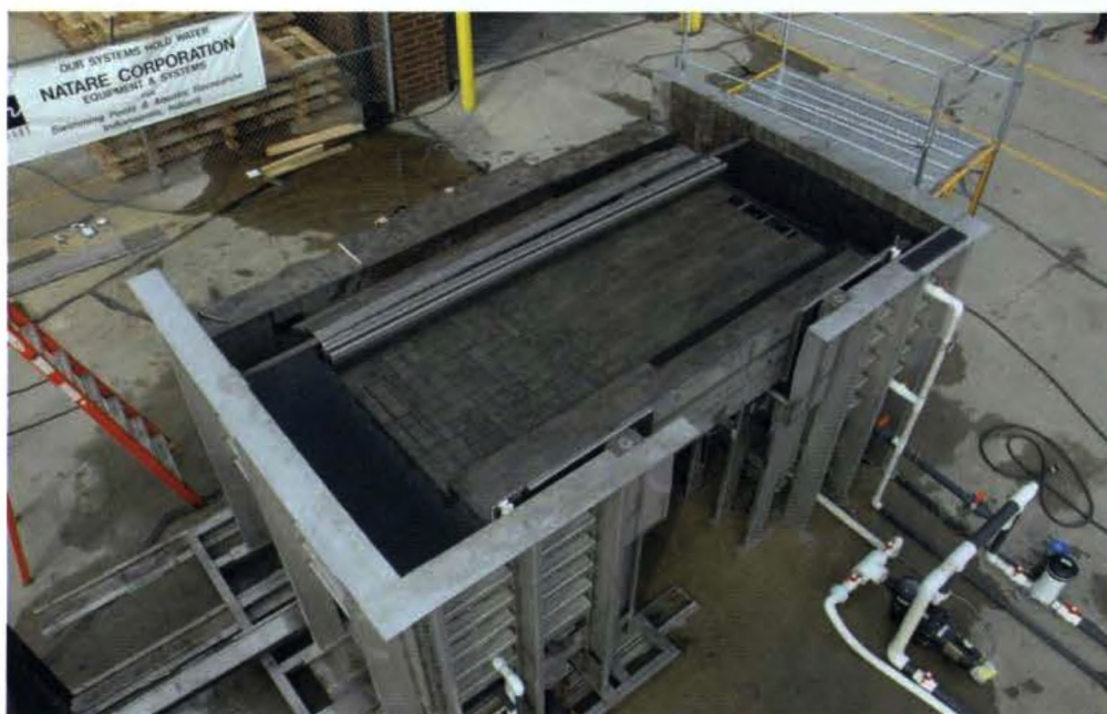
Figure 8. The pool's full scale mock-up for movement test
